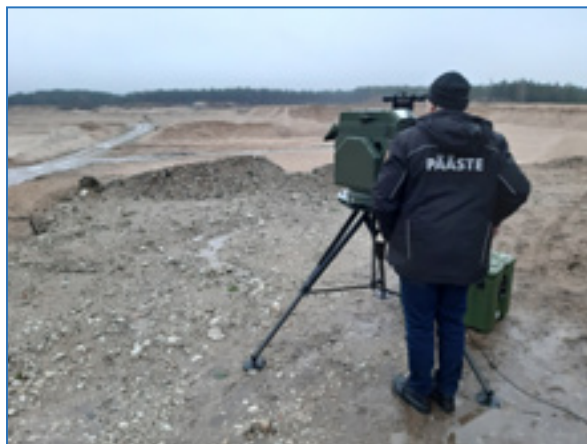
Fig. 2 • The Falcon 4G was positioned on a tripod and remotely controlled by an operator inside the vehicle.
